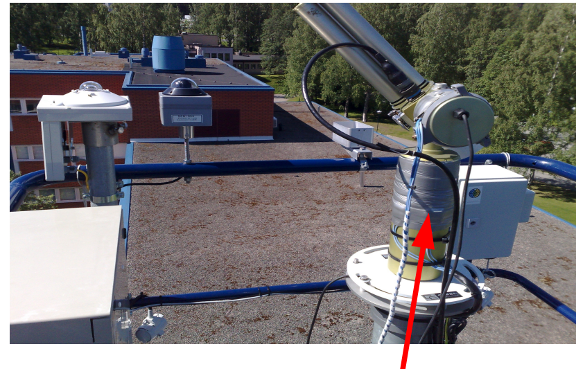
Sun photometer (Cimel) measuring in Kuopio site Finland June 2008
